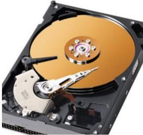
Figure 3.8: Inside of a hard disk drive
